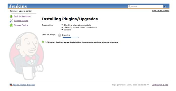
After restarting Jenkins, go to *Manage Jenkins* again, this time click on *Configure System* option and look for the TestLink section. Fill the TestLink configuration form with a name for your TestLink installation, the URL of the XML-RPC API and your *devKey*.
